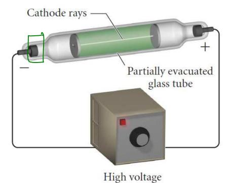
Cathode rays contain a single type of particle:
