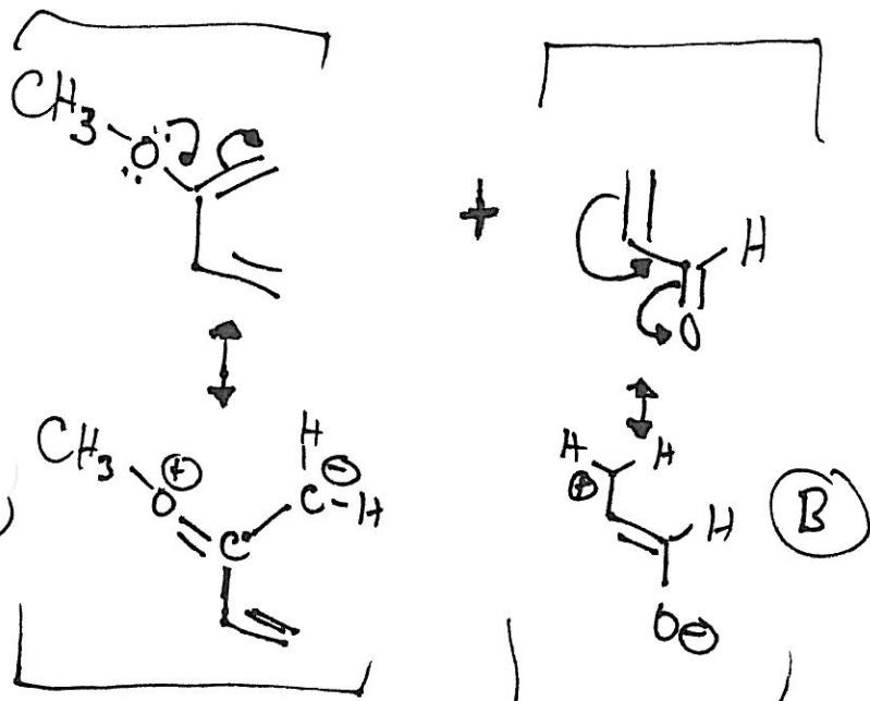
• In resonance structure **(A)**, the (-) end of the diene prefers to line up with the (+) end of resonance structure **(B)** (the dienophile). This orientation gives the 1,4 product.
